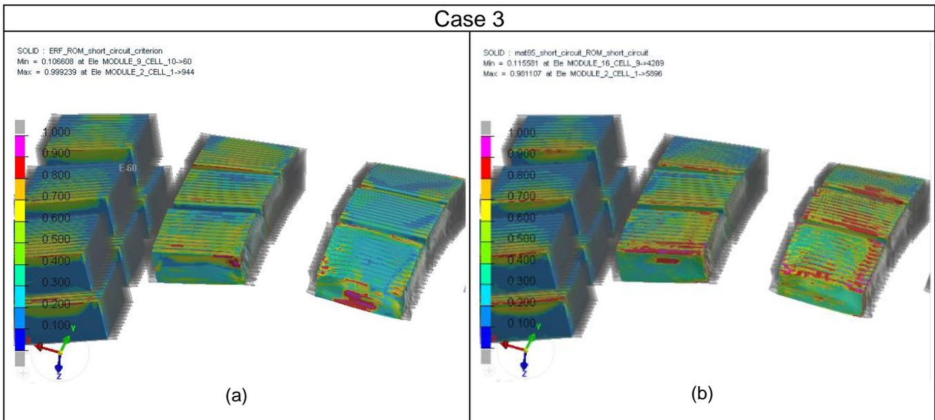
Figure 11: Homogenized material (a) and Plugin material (b) results comparison - Case 3 (Images taken at 100 ms)
