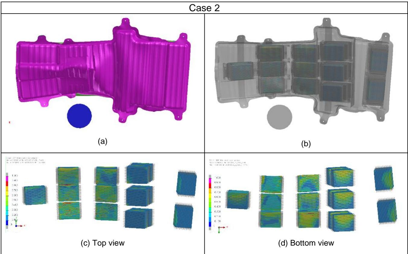
Figure 4: Homogenized material, Pole impact results - Case 2 (Images taken at 100 ms)
