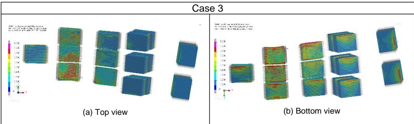
Figure 8: Plugin material, Pole impact results - Case 3 (Images taken at 100 ms)
