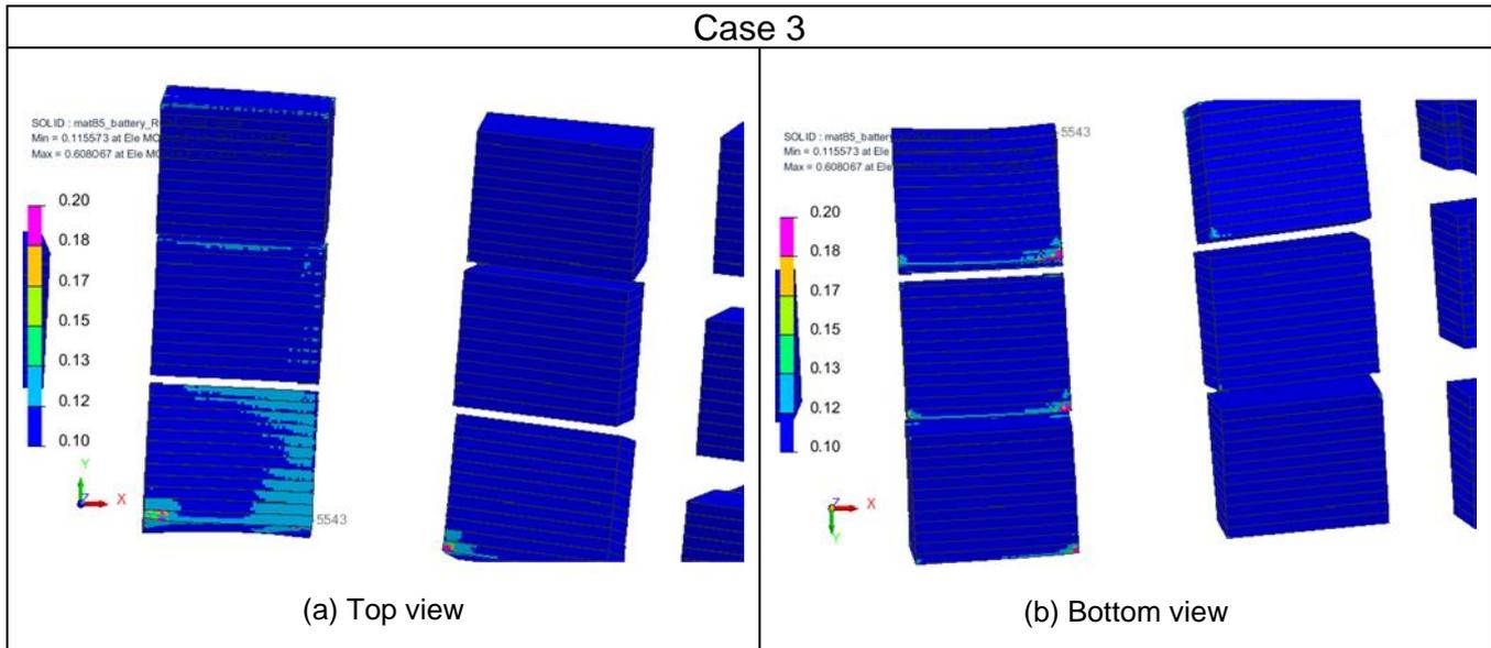
*Figure 16: TANN Plugin material, Pole impact results - Case 3 (Images taken at 100 ms).*
