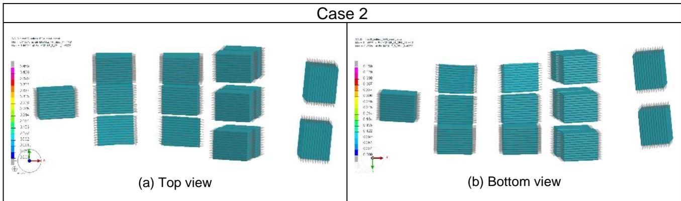
Figure 14: TANN Plugin material, Pole impact results - Case 2 (Images taken at 100 ms)
