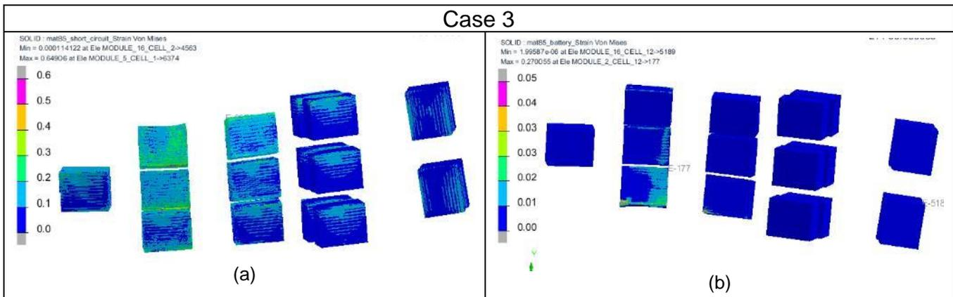
Figure 18: Von Mises Strain map with honeycomb material law (a) and with ROM stiffness material law (b), Pole impact results - Case 3 (Images taken at 100 ms).
