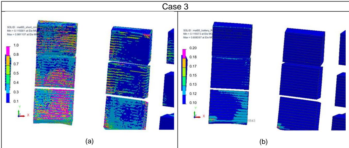
Figure 19: Short circuit risk with honeycomb material law (a) and ROM stiffness material law, Pole impact results - Case 3 (Images taken at 100 ms).
