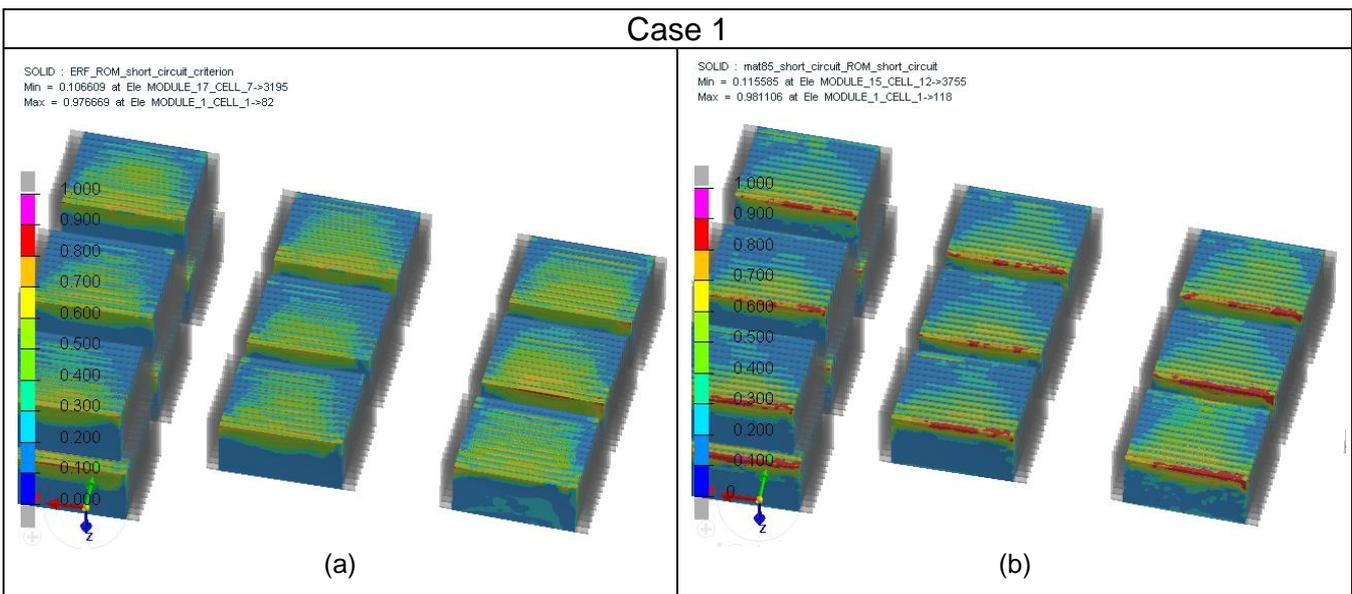
Figure 9: Homogenized material (a) and Plugin material (b) results comparison - Case 1 (Images taken at 100 ms)
