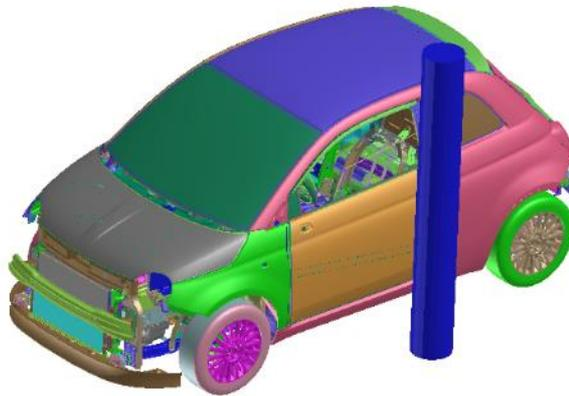
Figure 2: Side pole impact test
