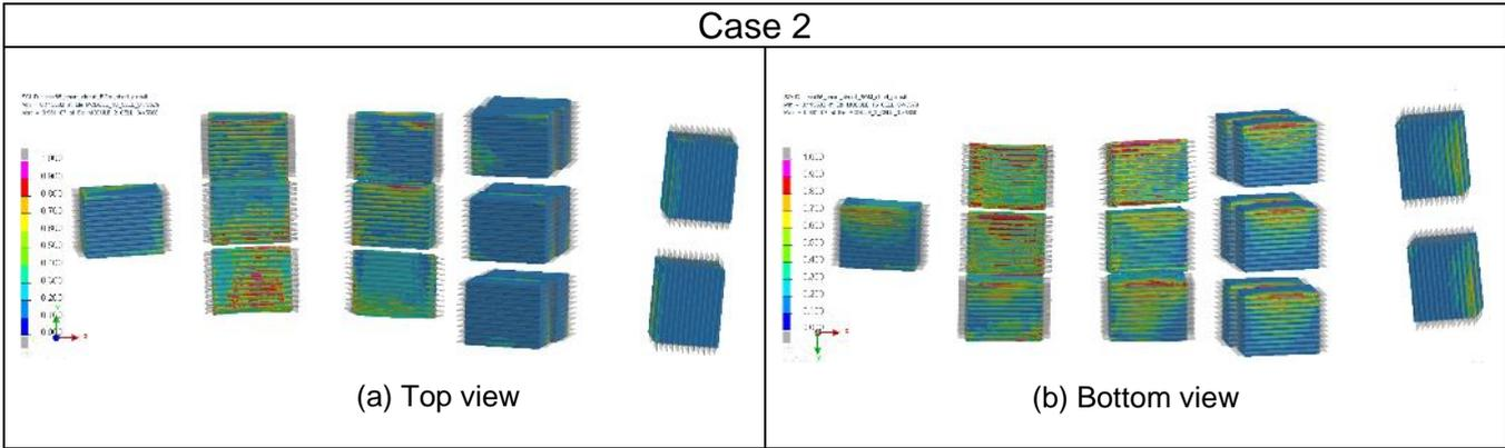
Figure 7: Plugin material, Pole impact results - Case 2 (Images taken at 100 ms)
