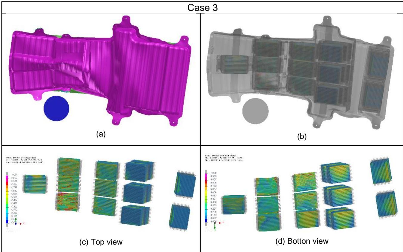
*Figure 5: Homogenized material, Pole impact results - Case 3 (Images taken at 100 ms)*
