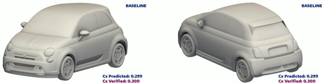
Figure 2: An animation of the geometry evolution through the optimization procedure. Fiat 500e.
